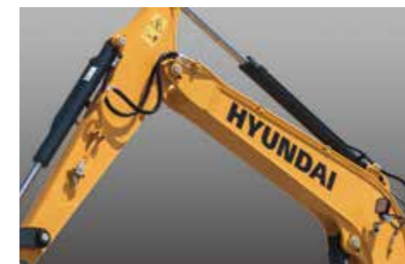
Standard breaker piping
