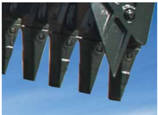
Horizontal type bucket pin
