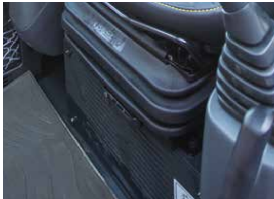
Air filter is located underneath the seat position for easy maintenance.
